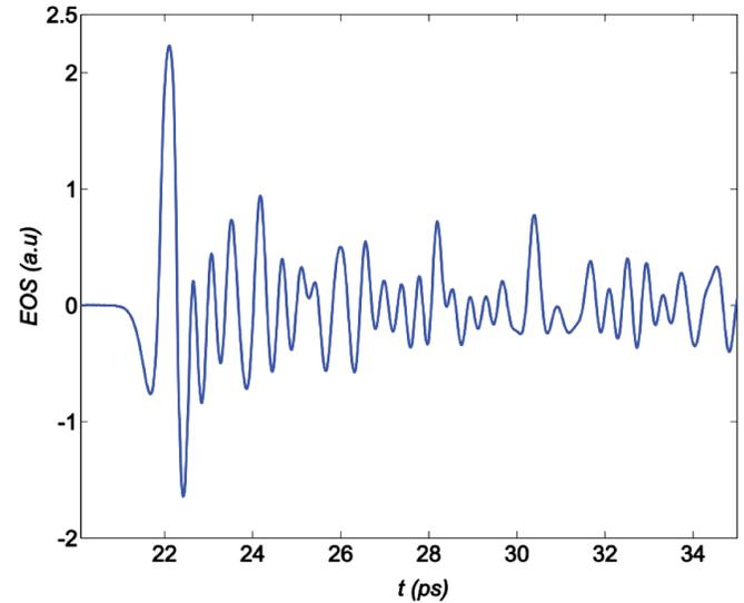
Fig. 3: THz signal versus time delay measurement (Courtesy of Fritz Haber Institute, Berlin, Germany)
