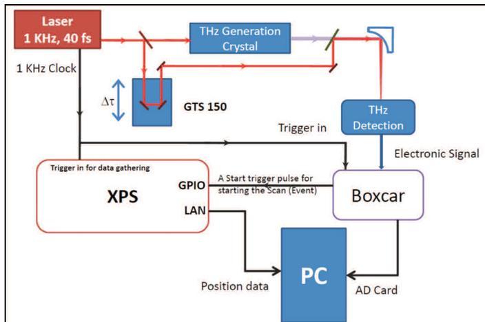
Fig. 1: Schematic of a THz scanning system (Courtesy of Fritz Haber Institute, Berlin, Germany)
