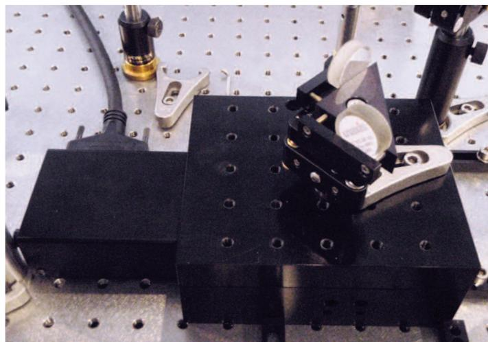
Fig. 2: Custom GTS70 high precision linear stage in the THz scanning system
