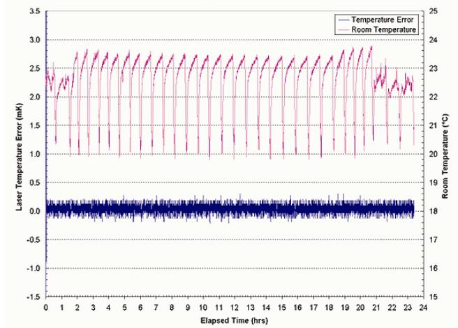
FIGURE 5 – Laboratory Environment Temperature Error
