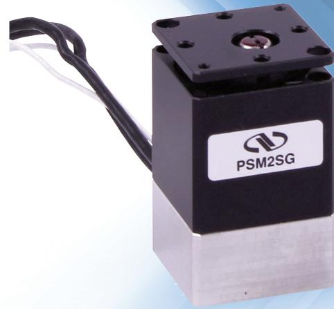
The PSM2 provides high-speed, sub-microradian resolution, tip, tilt, and z-motion for mirrors, gratings and other optics. Equipped with a direct piezo actuation system without lever arm transmission, the PSM2 is ideally suited for high bandwidth laser beam steering, switching and stabilization, beam scanning, image stabilization, and laser cavity tuning.
