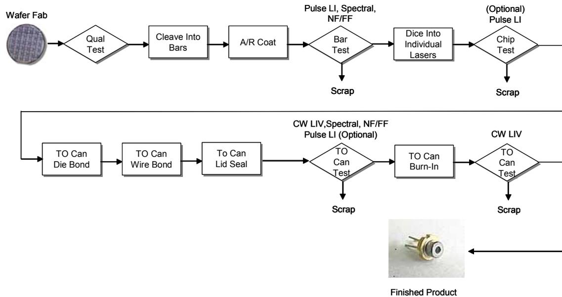
Figure 5 - Laser Diode TO-Can Packaging Line
