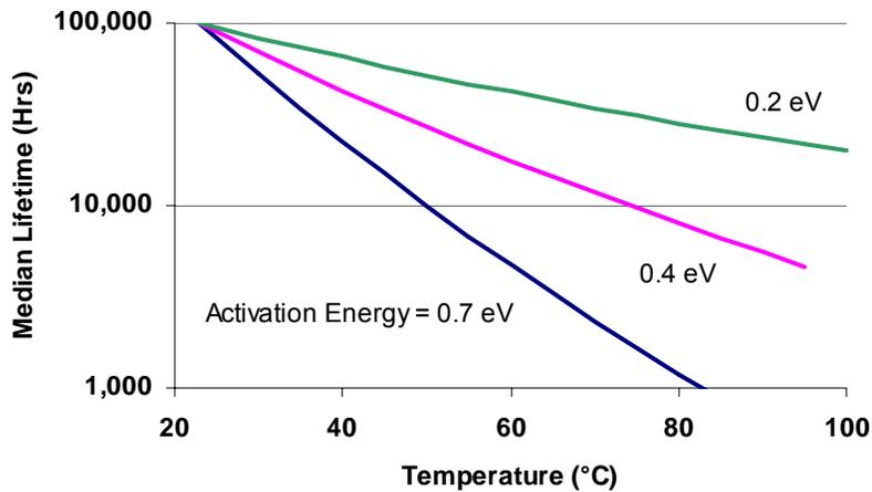
Figure 4 - Laser Lifetime Variation with Temperature
