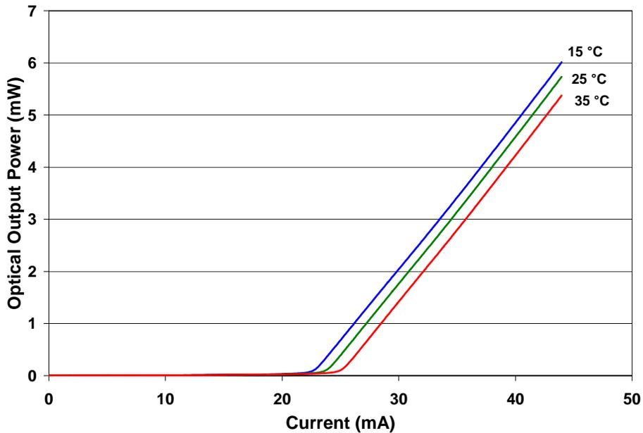
Figure 2 - Temperature Dependence of Light vs Current
