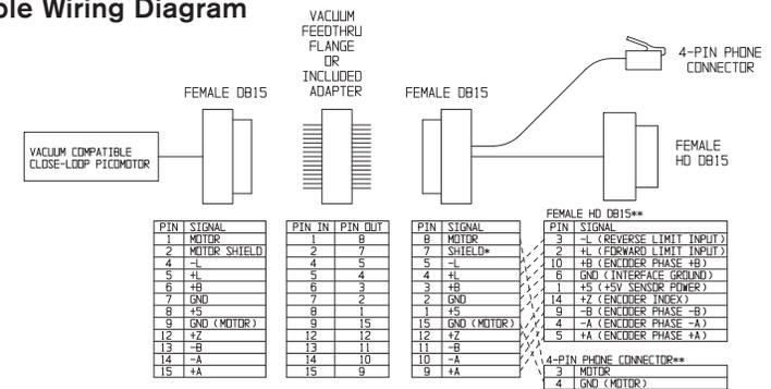
\*MOTOR SHIELD IN VACUUM CABLE IS TERMINATED TO THE CABLE SHIELD IN THE NON-VACUUM CABLE.
