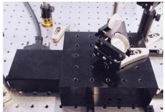
Fig. 3: Custom GTS70 high precision linear stage in the THz scanning system
