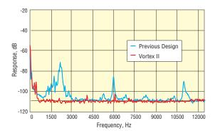
Frequency responce of Vortex II in compareson with original Vortex (100 dB white noise test). The Vortex II has improved stability due to the Star-Flex design and magnetic damping.
