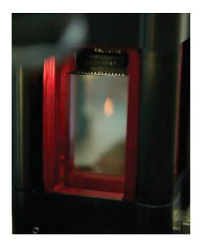
ColdQuanta's innovative BEC system is designed to streamline and simplify the production of ultracold atoms and BECs. At the heart of the system is the RuBECi® where rubidium atoms are cooled to temperatures of below 1  $\mu\text{K}$ , trapped, and manipulated inside the vacuum cell. A New Focus Tapered Amplifier is used to provide ample power for laser cooling and manipulation of the atoms.
