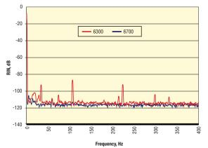
RIN test data for the Velocity 6700 and previous model Velocity 6300
