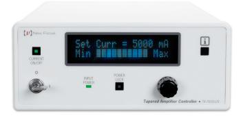
The VAMP TA is controlled using the TA-7600-LN Controller. Full control is made possible through the easy-to-use front panel interface. In addition, full control is also available using the USB or RS232 communication ports on the rear panel. Through the controller you can monitor the tapered diode temperature by way of a temperature sensor mounted on the diode block. Thermoelectric coolers are used to control the temperature of the diode.
