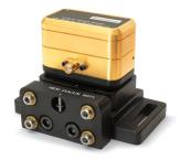
Aligning modulators is easy with the Model 9071 four axis aligner
