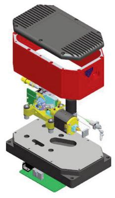
Mechanical schematic of the TLB-6700 laser platform
