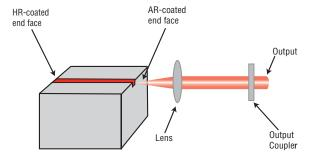
Figure 1. Laser diode placed into an external cavity.
