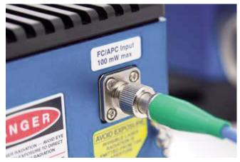
FC/APC input connector on the VAMP TA makes alignement a snap.
