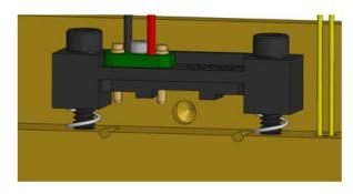
Figure 2.4 Laser Mounting Clamp with the Spring Contact Pins in the Left Position
