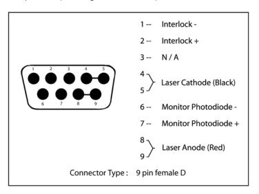
Figure 2.2 Laser Current Connector Pin Out
