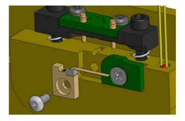
Figure 2.8 C-mount Laser Mounting
