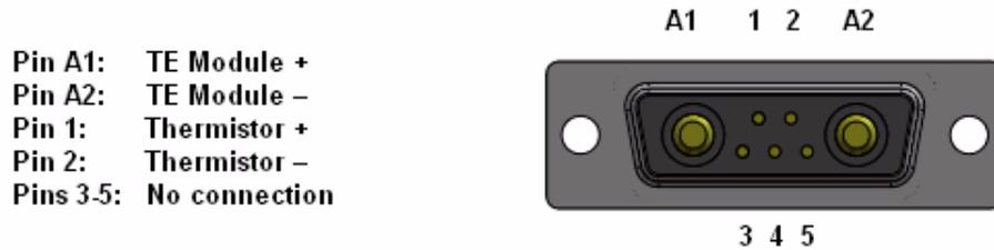
**Figure 2.3** Temperature Control Connector Pin Out
