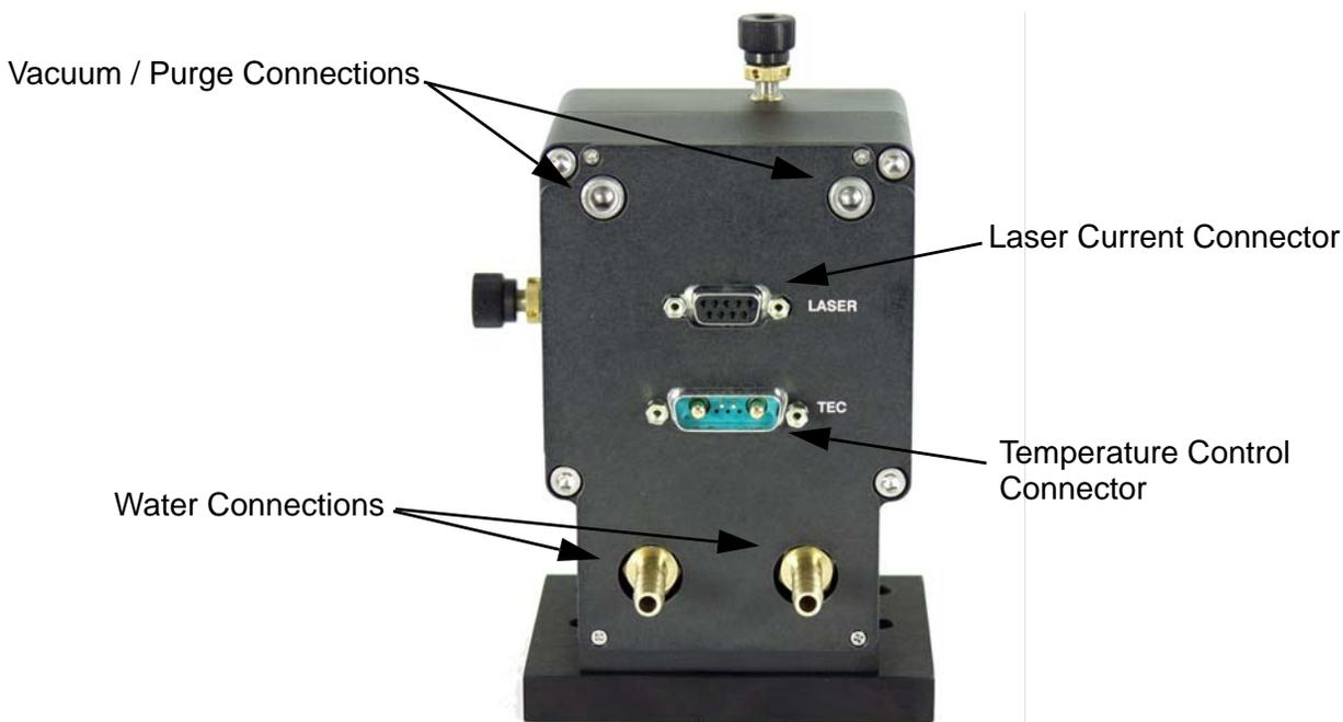
**Figure 2.1** LDM-487201 and LDM-487202 Rear Panel Connections
