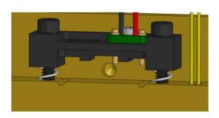
Figure 2.6 Laser Mounting Clamp with the Spring Contact Pins in the Right Position
