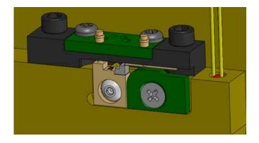
Figure 2.9 Correctly Installed C-mount Laser
