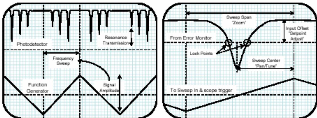
Figure 4: Typical oscilloscope signals are shown for locking to the side of an optical resonance. The dashed horizontal lines indicate ground for denoted signals. a) A triangle
