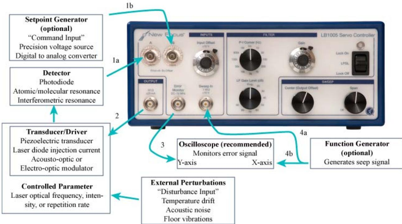
Figure 3: Typical signal connections for LB1005
