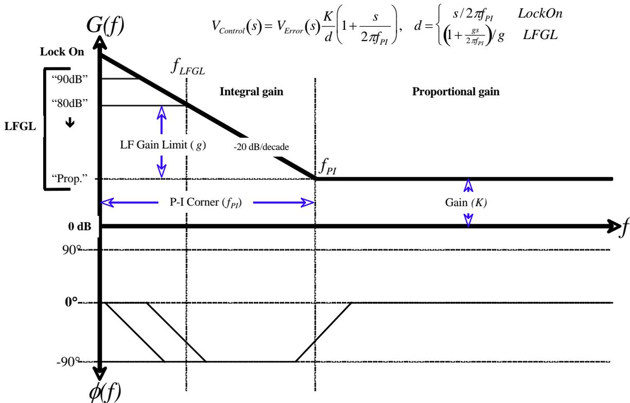
Figure 8: Proportional-integral Filter Gain with Low Frequency Gain Limit
