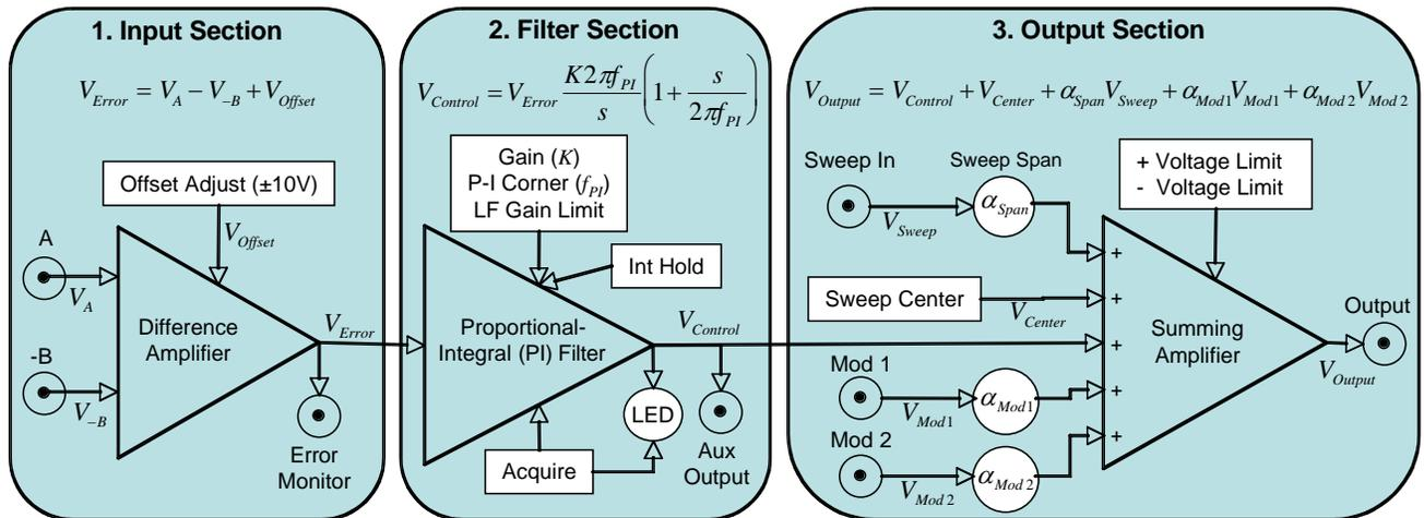
Figure 7: Schematic of LB1005 Signal Architecture
