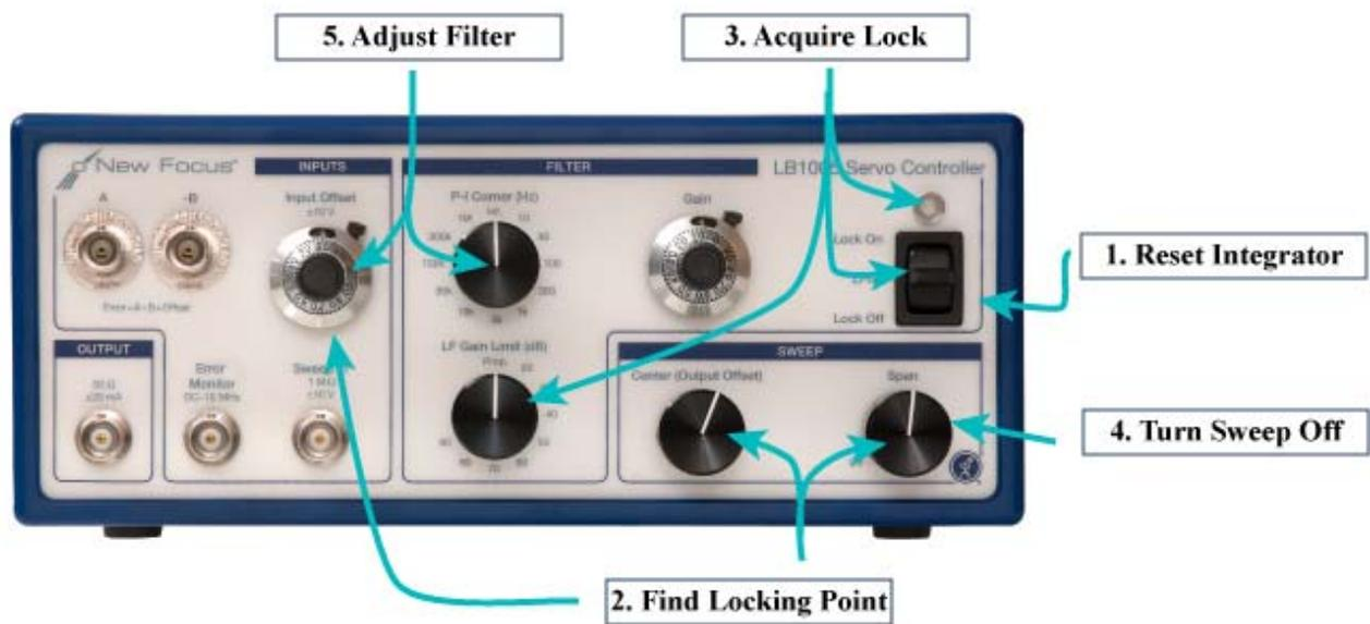
Figure 5: Typical Operation of Controls
