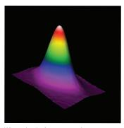
When using the free-space version, you can count on an excellent beam profile due to our post-amplifier beam shaping. Beam profile measured at 60 cm.
