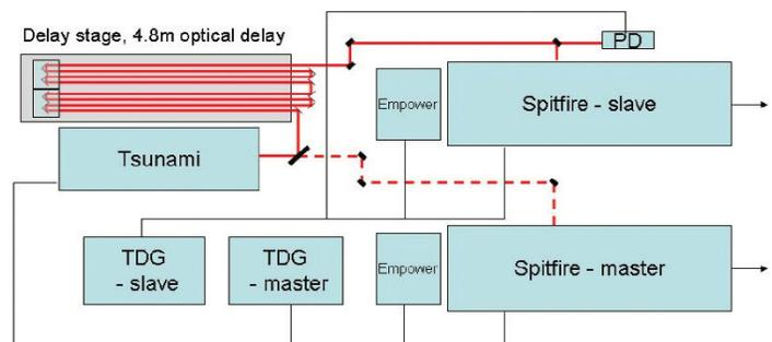
Fig. 1. Block diagram setup for synchronizing two amplifiers with a single oscillator. PD - photodiode; TDG - time delay generator.
