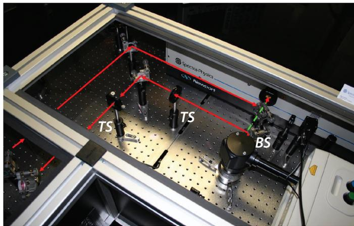
Figure 2. Beam routing at the Tsunami oscillator output. The seed beams for master and slave amplifiers are also shown by green dashed and solid red lines, respectively. BS - beamsplitter; TS - telescope set.
