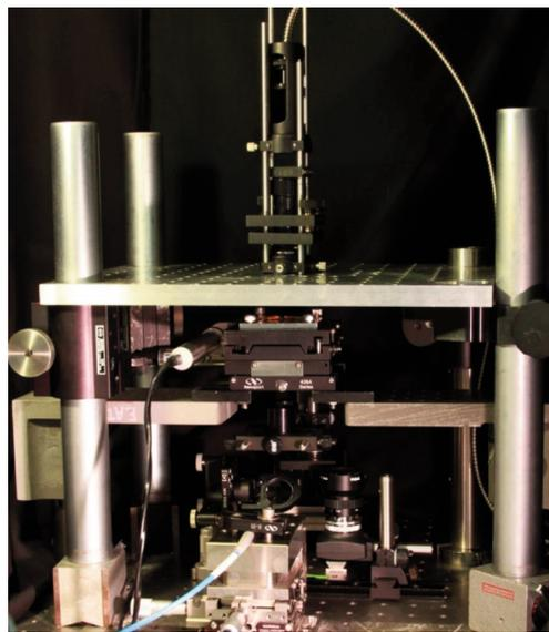
Figure 3: The experimental setup of Photonic Crystal Resonator Tester at Stanford, featuring stacked aperture stages with integrated actuators controlled by NSTRUCT (courtesy of Meredith M. Lee, PhD candidate)
