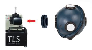
For photonic sensor characterization, a uniformly illuminated, flat field of light projected onto the active area of the sensor is vital for achieving accurate measurements. Newport's line of integrating spheres optimizes the output light of the TLS for sensor characterization applications. The SPH-UAPT is necessary for coupling the TLS output to an integrating sphere with 1.0 inch diameter port. See our website for coupling adapters suitable for other diameter ports.
