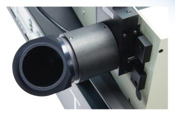
The 1.5 inch output flange of the TLS260 is an optical assembly incorporating a protected aluminum coated mirror. This mirror's off-axis replicated parabolic design features the focal point displaced from the mechanical axis, eliminating the typical shadow effect observed when a detector or light source is placed at its focal point. The output flange has 360° freedom of rotation, providing flexibility and convenience in installing the TLS260 into existing measurement systems.
