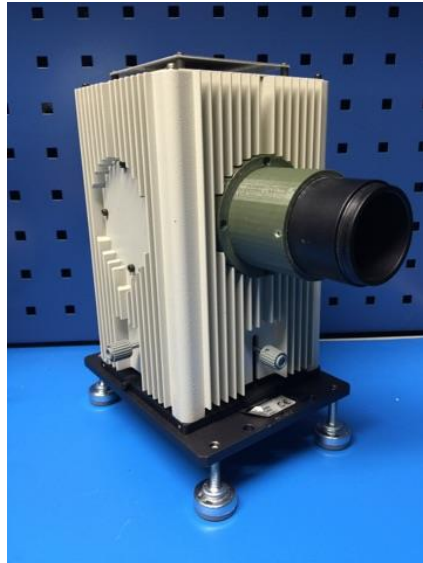
Figure 4: Light shield extension tube mounted.
