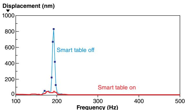
FIGURE 1. The magnitude of movement that can be experienced by an optical mount in a typical lab environment when subject to broadband noise is influenced greatly by the damping capabilities of the optical table on which the mount sits.
