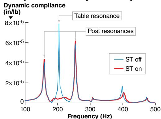
FIGURE 3. The influence of active damping of a table on transfer dynamic compliance from the table to the top of the post. Transfer dynamic compliance estimates the ratio of the horizontal acceleration on the top of the post (recalculated into displacement) to the vertical force on the table, as a function of frequency.
