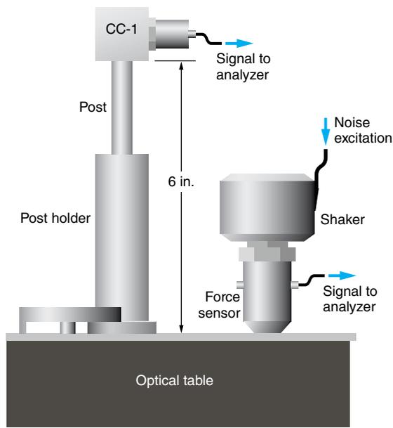
FIGURE 2. A test setup measures the transfer function from a tabletop force into the horizontal motion on the tip of an optical mounting post. (Courtesy of Newport)
