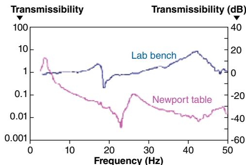
FIGURE 4. Vibration transmissibility of vertical floor motion is greatly improved with a Newport pneumatic isolation workstation compared to a typical built-in laboratory bench. (Courtesy of Amick and Stead, *Meeting of the ASA*, 2002)
