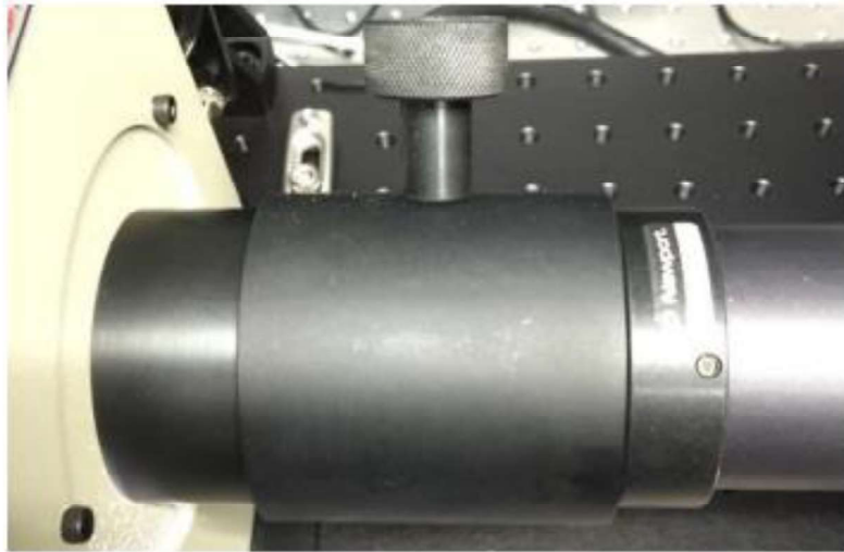
Condenser lens assembly adjustment knob and adjustment lever at output of lamp housing
