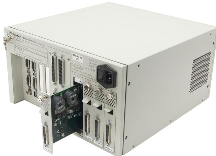
*Figure 6: Installing driver cards.*
