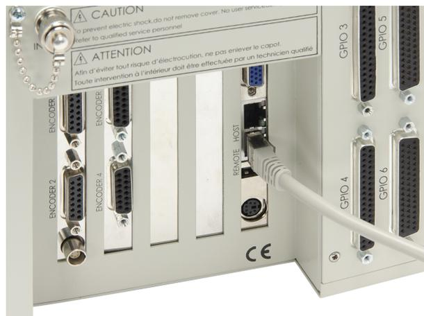
*Figure 10: Direct connection to the XPS-RL using a cross-over cable and the REMOTE connector.*
