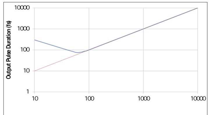
**Figure 3.** Broadening of a femtosecond pulse at ~ 1050 nm after propagation through 8 mm of TGG (blue curve); the red curve shows the output for undistorted pulses.
