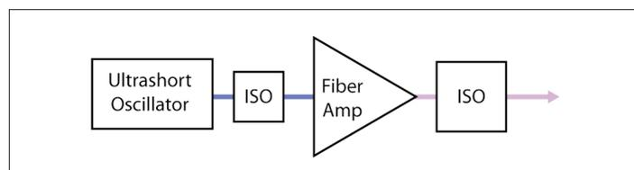
**Figure 2. Typical CPA Design, showing the use of isolators (denoted ISO) and their locations in the beam path.**
