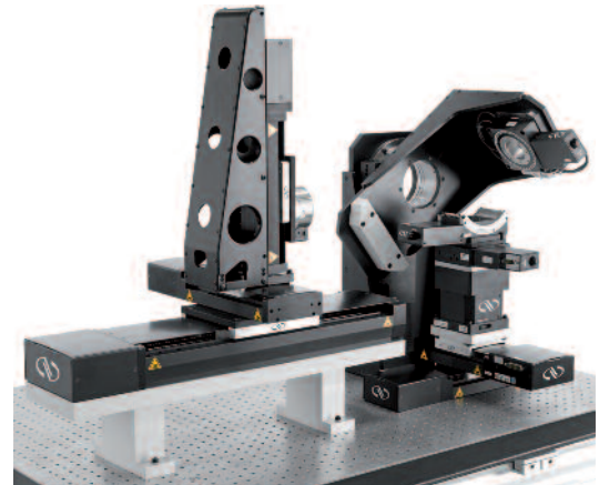
Figure 3: 11-Axis Motorized System for Calibration of On-Vehicle Safety Sensors
