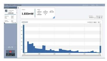
PMManagerApplication Window, with Histogram plot of only one channel
