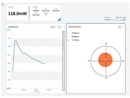
The above image shows the PEPS sensor displayed in Track w/Power mode as the orange Position graph and power from another sensor as the Line graph in blue.
