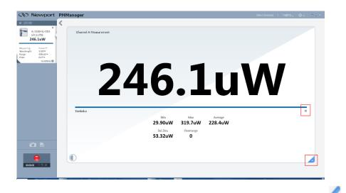
To fill the entire screen area with the expanded view of the numerical area, click the sicon, in the display area. Click the appropriate button(s) to return to default size.
