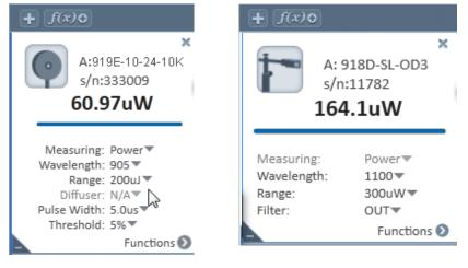
Pyroelectricsensor Measuring mode and parameters Photodiode sensor Measuring mode and parameters
