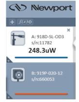
The channel measurement frame displays the current value measured by the sensor, adjusted by enabled (if any) Function parameters.
