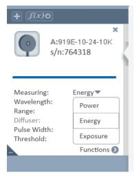
The pyroelectric screen fields displayed depend on the mode selected.
