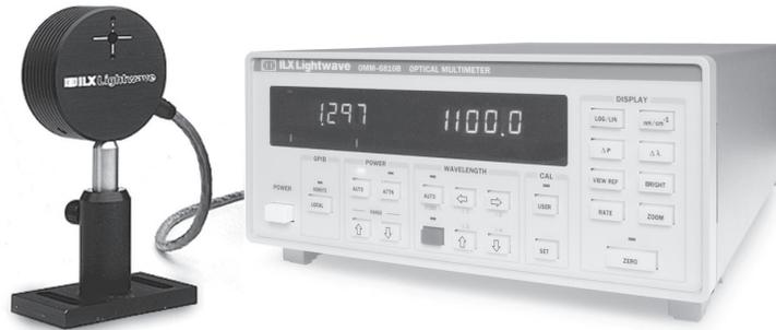
back reflection. Integrating spheres are inherently insensitive to beam profiles, providing you with more flexibility in laser type and launch conditions. Filtered detectors on the interior of the sphere receive an equal distribution of incident light, ensuring that the calibration and resultant measurement accuracy are independent of the beam profile.
