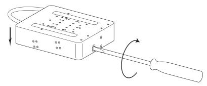
③ Inset one of both screw guides supplied in both mounting holes located on the cable output size of the stage, until the guide end is in contact with the bottom of the countersink receiving the mounting screw in the base. Slip one CHC M4 screw (not supplied) into each screw guide and screw it until the headscrew is in contact with the bottom of the countersink.
