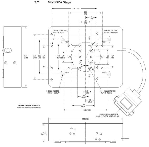
Components with counterbored holes for M6 screws can be attached to the top plate of the M-VP-5ZA using M4 and the washers supplied with each stage.
