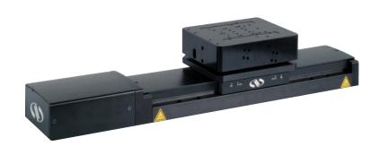
A VP-5ZA stage mounted on top of an ILS linear stage (with optional VP-BP base plate). The vertical lift approach of the VP-5ZA allows centering of the payload over the bearings and close to the position feedback system. This avoids any cantilevered loads and results in more precise motion with higher load capacity.
