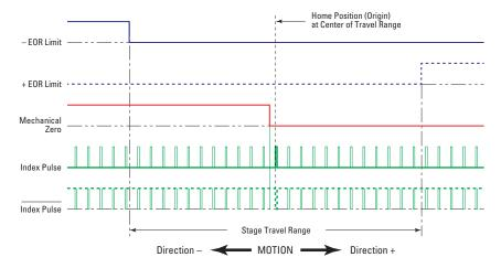
End-of-Run and Mechanical Zero are 5 V open collector type. The Index Pulse provides a repeatable Home Position at ±1 step.
