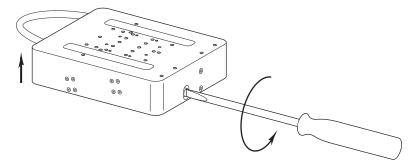
6 Repeat step 3 for both mounting holes located on the manual knob size of the stage. Tighten both mounting screws at the nominal torque.
