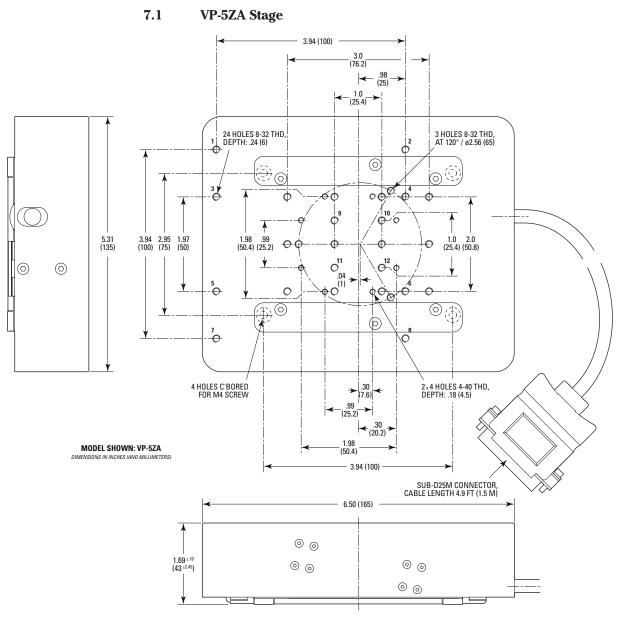
Components with counterbored holes for 1/4-20 screws can be attached to the top plate of the VP-5ZA using 8-32 and the washers supplied with each stage.
