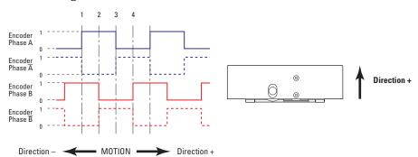
The incremental sensor consists of an optical scale and an encoder head. When the carriage moves, the encoder head generates square signals in
