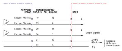
"Encoder" are "differential pair" (type RS-422) type output signals. Using these signals permits a high immunity to noise. Emission circuits generally used by Newport are 26LS31 or MC3487. Reception circuits to use are 26LS32 or MC3486.
