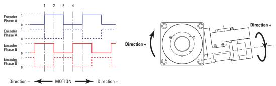
The incremental sensor consists of an optical scale and an encoder head. When the carriage moves, the encoder head generates square signals in quadrature and sends to pins #6, #7, #13 and #14 of the SUB-D15 connector.
