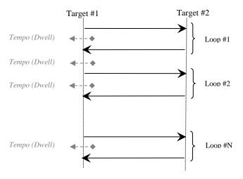
In the "Target position / PA-Move Absolute" area, two target positions can be defined. The "Go to" button executes the absolute move to the specified target position.
