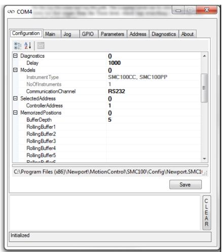
The polling interval defines the number of milliseconds between each time the Controller GUI polls the SMC100 for the latest information. The user may change the polling interval by entering a value. Diagnostics Delay defines the time delay in milliseconds between each command sent from a text file. InstrumentType and NoOfInstruments display the type of controller and number of the connected instrument.
