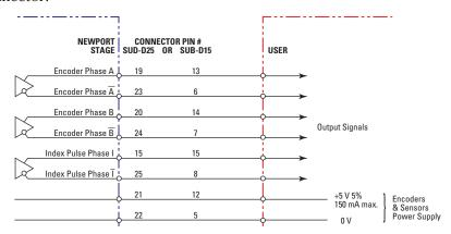
"Encoder" and "Index Pulse" are "differential pair" (type RS-422) type output signals. Using these signals permits a high immunity to noise. Emission circuits generally used by Newport are 26LS31 or MC3487. Reception circuits to use are 26LS32 or MC3486.
