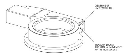
At the end of the drive screw of the RV Series stages (side opposite motor), a hexagon socket is given for manual movement of the mobile core, using an "Allen" wrench.
