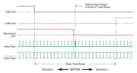
End-of-Run and Mechanical Zero are 5 V open collector type.
