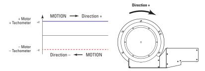
In the above drawings, + Motor signal is referred to – Motor signal, + Tachometer signal is referred to – Tachometer signal.
