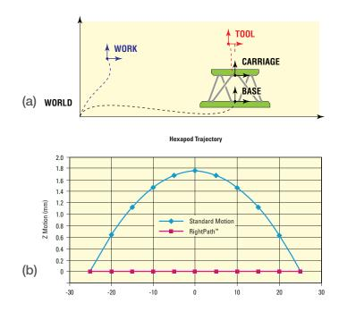
Figure 5. (a). MKS Instruments' HXP hexapod Work and Tool coordinate systems transformation of axes; (b) RightPath™ trajectory showing runout.
