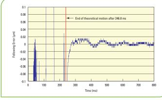
Figure 3. Step and settle characteristics of an MKS linear motion stage 250 ms after being moved.
