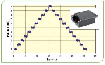
Figure 2. 1 nm MIM of an XMS linear stage; Insert – MKS Instruments' XMS50-S Linear Motor Stage.
