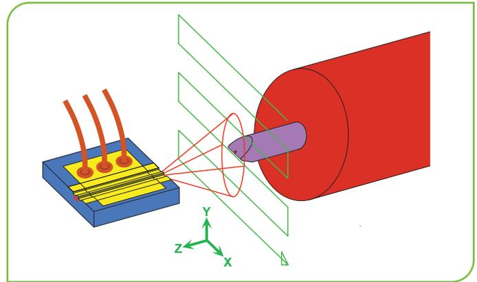
Figure 1. The operations and positional parameters of optical fiber alignment; (a) scan operations; (b) positional parameters for the optical fiber alignment.
