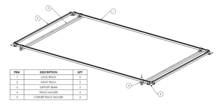
Use as many people as needed to flip and lift frame assembly. Adjust positions of support beams as needed and set support beams on top of vertical mounting bracket that you previously installed.
