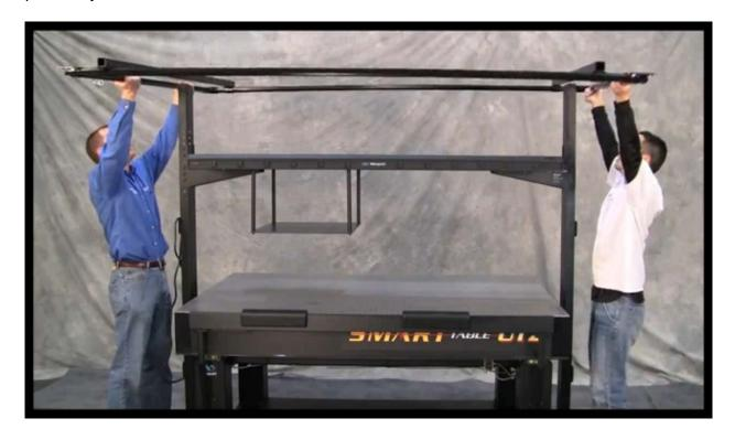
Attach support beams to vertical bracket. There are two sets of holes to accommodate different shelf locations.
