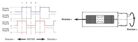
The incremental sensor consists of an optical scale and an encoder head. When the carriage moves, the encoder head generates square signals in quadrature and sends to pins #19, #20, #23 and #24 of the SUB-D25 connector.
