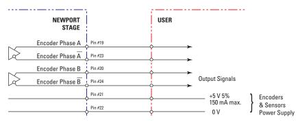
"Encoder" are "differential pair" (type RS-422) type output signals. Using these signals permits a high immunity to noise. Emission circuits generally used by Newport are 26LS31 or MC3487. Reception circuits to use are 26LS32 or MC3486.
