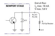
To enable End-of-Run, when a MFA stage is used with non-Newport controllers using the Sub-D25M connector provided, pin #13 must be connected to +5 V with a pull-up resistor (ex: 4.99 k $\Omega$ ).
