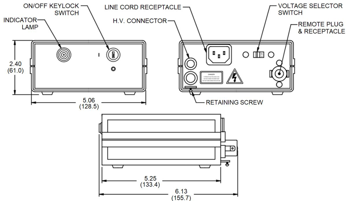
Standard Configuration for Laser Heads N-LGx-193, 393
