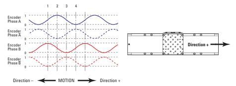
The incremental sensor consists of an optical scale and an encoder head. When the carriage moves, the encoder head generates sine-cosine signals in quadrature, sent to pins #1, #3, #9 and #11 of the SUB-D15 connector.
