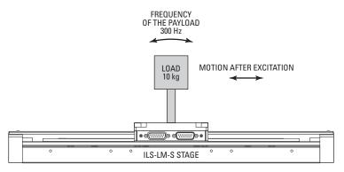
Driving in force requires a good adjustment of the controller/driver theoretical acceleration parameter (ScalingAcceleration) which depends on the moving mass.
