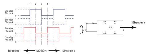
The incremental sensor consists of an optical scale and an encoder head. When the carriage moves, the encoder head generates square signals in quadrature and sends to pins #19, #20, #23 and #24 of the SUB-D25 connector.
