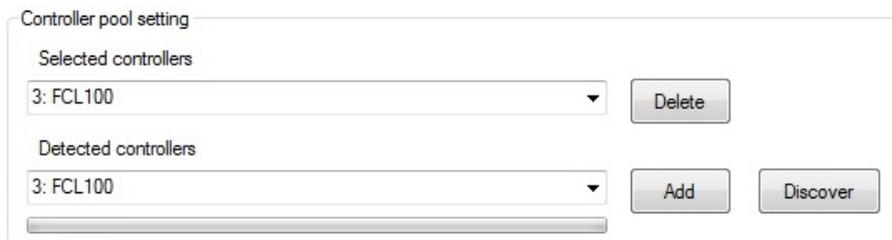
After a *Discover* action, the list of detected controllers is filled. Stage model number is shown next to the address #1 through #4. This address helps to identify each controller connected.
