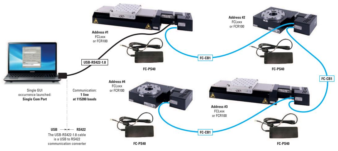
Each stage from the chain must have a different address from 1 to 4 (default is 1).
