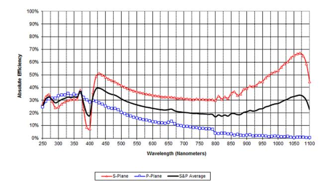
**Note:** The efficiency curve above is absolute and was measured in an in-plane near Littrow configuration (unless otherwise indicated). Efficiency curves are only representative: actual efficiency may vary significantly depending on use geometry and measurement technique. This efficiency curve is for master 5469; two masters with the same catalog number may have different efficiency curves. The uncertainty band on the data in the above efficiency curve(s) is +/- three percentage points.
