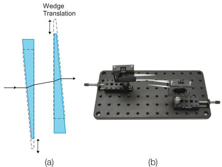
**Figure 7.** (a) Beam propagation through a pair of identical wedges. The translation of the prism allows the continuous tuning of positive GDD while avoiding angular deviation. (b) Experimental implementation which includes Newport's 25RB12-01UF.AR2-M mounted wedges, HVM-1i top adjust mirror mount, SP-1, 1" optical mounting post, SPH-1 slim optical post holder, 422-1S miniature ball bearing stage, TR-8Q20 adaptors 1/4-20 to 8-32 thread, all mounted on the SA2-06x12 aluminum optical breadboard.
