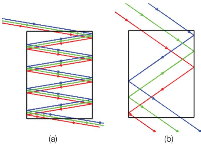
**Figure 6.** Zemax simulations for a pair of reflective surfaces separated by 15 mm as a function of beam diameter and angle of incidence for: (a) 2 mm, 9.5° and (b) 6 mm, 35°.
