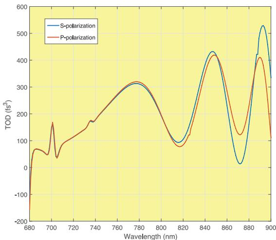
**Figure 4.** Theoretical third order dispersion (TOD) for Newport 10Q20UF.40 ultrafast multi-layer dielectric coating chirped mirror for a 5° angle of incidence. The chirped mirror delivers no more than 500 fs<sup>3</sup> TOD (cubic term) across the 680 to 900 nm wavelength range.
