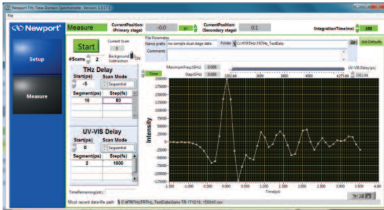
Software showing acquisition of time resolved THz data for gallium arsenide
