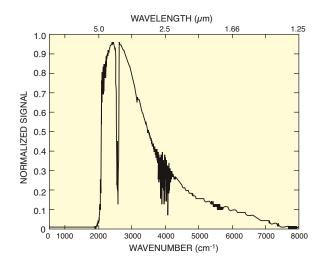
Fig. 7 Spectrum of 1273 K blackbody captured with 80021 InSb Detector,  $\text{CaF}_2$  beam splitter and the 8035TM Scanner
