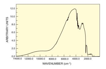
Fig. 8 Spectrum of 80009 QTH Source taken by 8035 with a  ${\rm CaF_2}$  beam splitter and 80008 DTGS Detector
