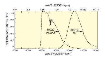
Fig. 4 Spectrum of 1273 K blackbody captured with InGaAs and Si Detectors,  ${\rm CaF_2}$  beam splitter and the 8035 scanner
