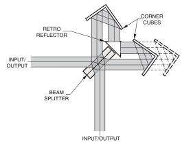
Fig 2. Optical layout includes corner cubes and a retro-reflector mounted to a beam splitter
