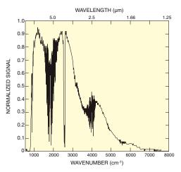
Fig. 6 Spectrum of 1273K blackbody captured with the 80026 MCT Detector, KBr beam splitter and the 8035 Scanner.
