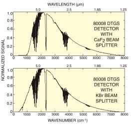
Fig. 5 Spectrum of 1273 K blackbody captured with 80008 DTGS Detector,  $\rm CaF_2$  beam splitter was used to acquire the top measurement; a KBr beam splitter was used for the bottom measurement.
