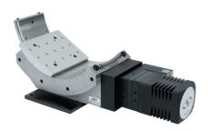
**Note:** To access the interface holes of the carriage, simply move the bottom stage to its extreme position. Two c'bored holes will be accessible from one end of travel and the other two holes will be accessible from the other end of travel. For example, between the BGM160 and BGM200, use the M6 holes in a 6.14 x 3.62 (156 x 92 mm) pattern. BGS80 on BGM120, use M4 holes in a SQR 1.89 (48 mm) pattern.
