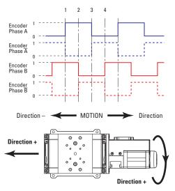
The incremental sensor consists of an optical scale and an encoder head. When the carriage moves, the encoder head generates square signals in quadrature and sends to pins #19, #20, #23 and #24 of the SUB-D25 connector or pins #6, #7, #13 and #14 of the SUB-D15 connector.
