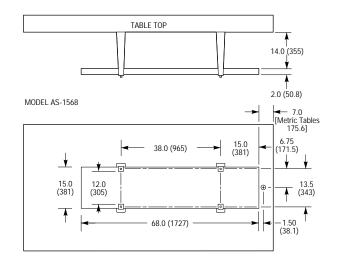
Figure 2.1 — Mounting Post Location
