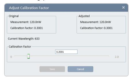
The **Original** area displays the original **Measurement** and **Calibration Factor**.
