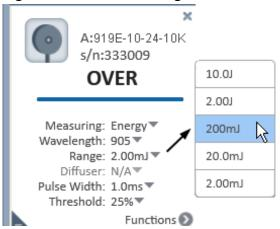
While measuring pulsing lasers, an erroneous energy reading will result if the energy range is not set up correctly.
