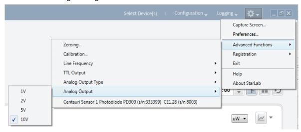
The analog output is driven through an impedance of 100 ohm. For best accuracy, it is recommended to limit the external load to 100K (or larger). A smaller load (down to 1K) is possible but may result in loss of accuracy.
