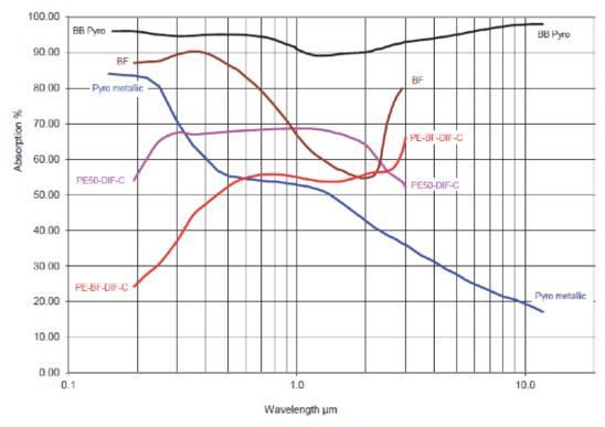
Absorption of Newport Pyroelectric Absorbers Absorption (%) vs. Wavelength (nm)
