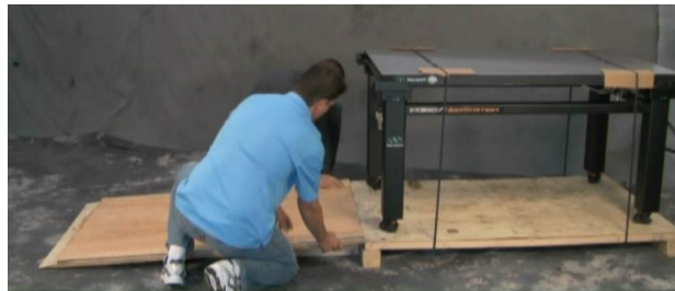
Figure 4 Vision IsoStation “roll off” ramp installation
