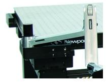
A long M6 screw (about 2.5 in.) is needed in order to secure the rod to the corner bracket. Insert the screw from the bottom of the corner bracket piece and apply enough torque to secure the rod on top of the corner bracket.
