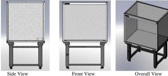
The four mounting blocks that come with the faraday cage are needed only if the extension shelves are attached to the workstation. They extend from the edge of the corner bracket so that users can mount extension shelves with the presence of faraday cage.
