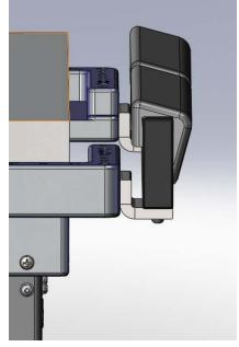
For 4" breadboard Vision IsoStation, the L shaped bracket should be flipped to make the hip guard position higher to match the height of the table top.
