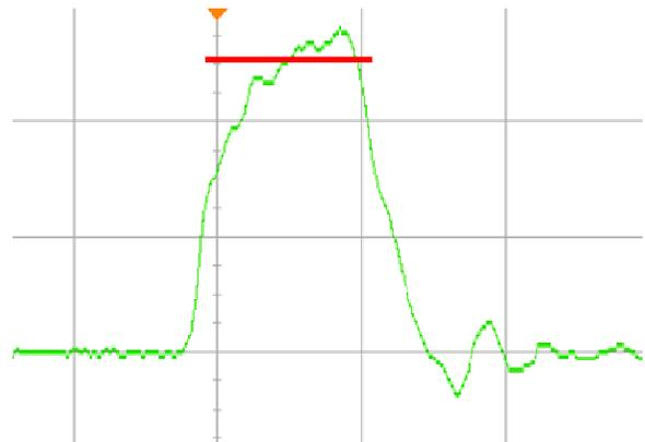
Figure 3: Waveform of 2.5 A, 25ns pulse, inductive load with the scope configured to 20 ns/division and 1 A/division
