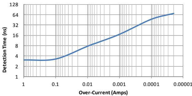
Figure 2: Secondary current limit Detection Time vs Over Current condition
