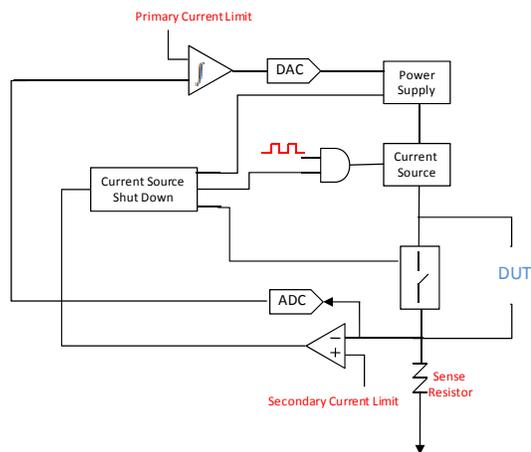
Figure 1: Current Limit Circuit Diagram
