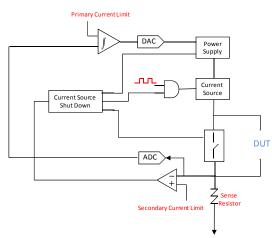
Figure 1: Current Limit Circuit Diagram
