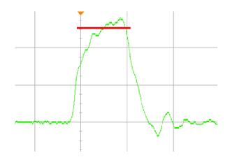
Figure 3: Waveform of 2.5 A, 25ns pulse, inductive load with the scope configured to 20 ns/division and 1 A/division
