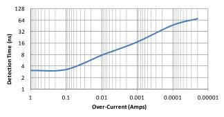
Figure 2: Secondary current limit Detection Time vs Over Current condition
