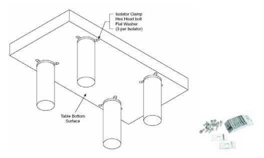
Figure 2 — Isolator Clamps and Mounting Holes
