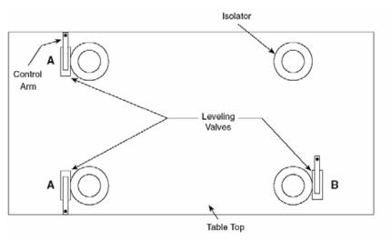
Figure 7 — Orientation of Control Arm
