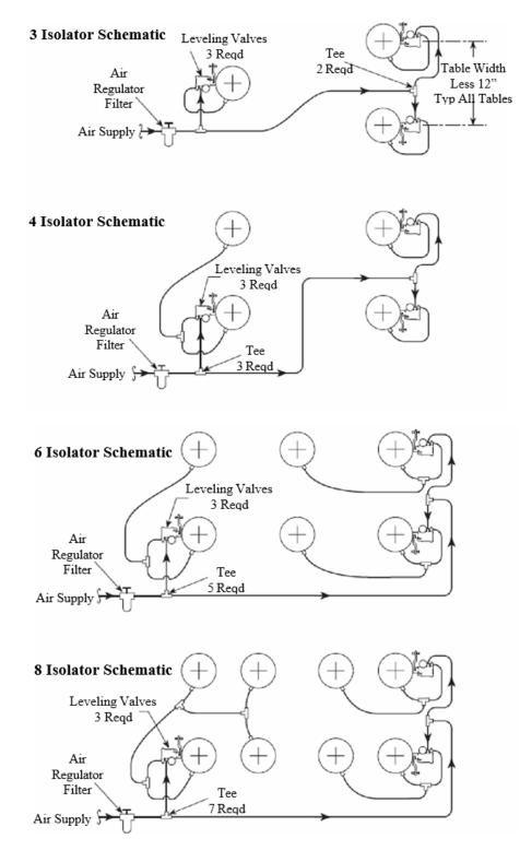
Figure 8 — Air Line Routing
