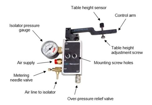
Figure 5 — IPV Leveling Valve
