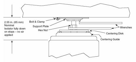
Figure 4 — Level Adjustment of Isolators
