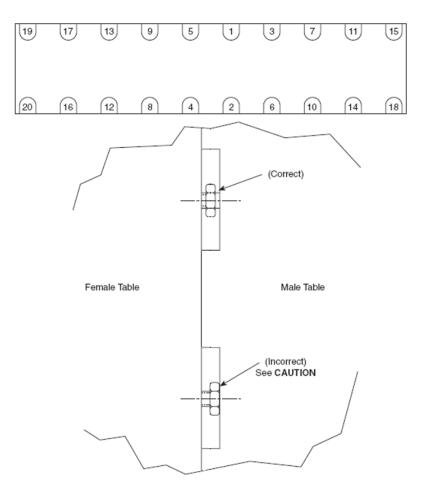
Figure 13 — Double Bolt Tightening Sequence
