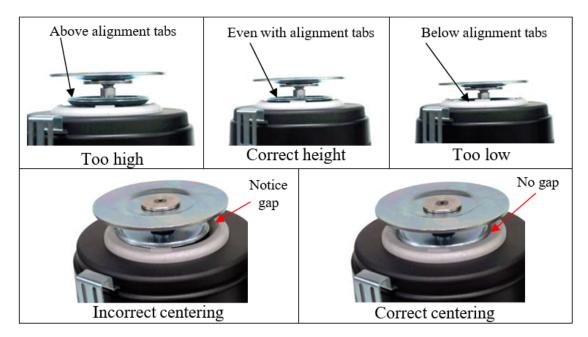
Figure 11 — Floating Height Adjustment and Centering
