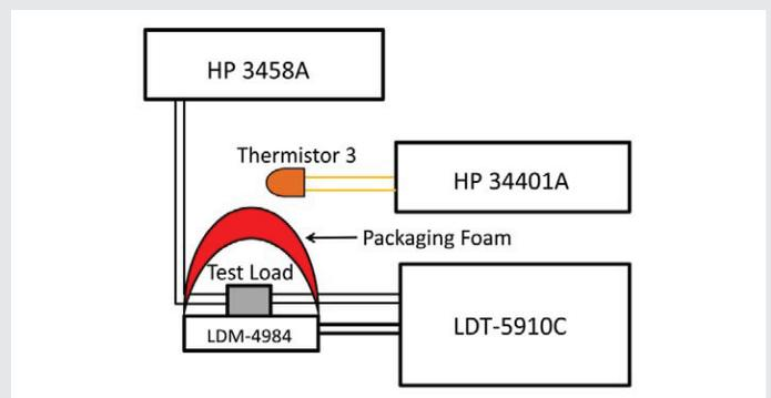
Figure 2: The temperature stability test setup.
